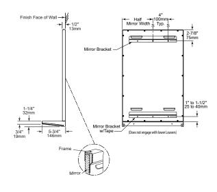
Note: Mirrors greater than 36" in width will have multiple hanger bracket pockets with a typical 8" off each edge.
